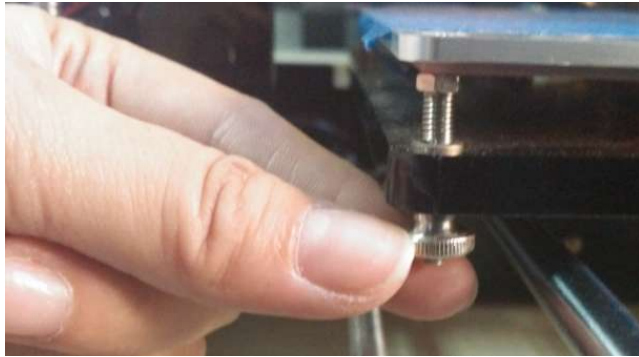
Fig 11: Adjust Print Platform Height
