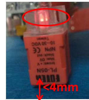
Fig 2: PS Trigger Height
